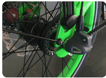
Internal Nexus 3 Speed Hub and Bell Crank
