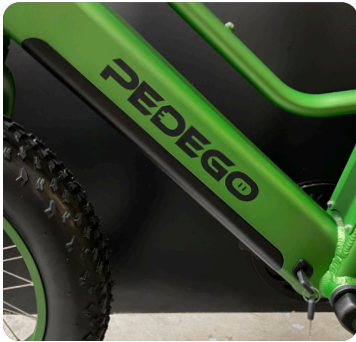
Battery Fully Installed
