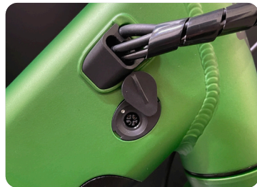
48v Charging Port
